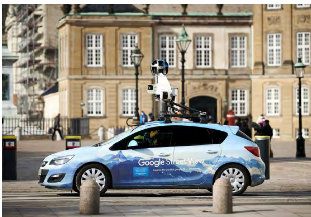
Google Street View car, fitted with advanced air quality measuring. ©Utrecht University
